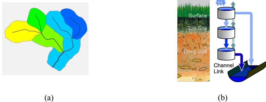
Figure 1.1 (a) illustration of landscape decomposition into hillslopes and decomposition of the river network into channel link and (b) vertical soil profile and control volumes included in the hydrological model
